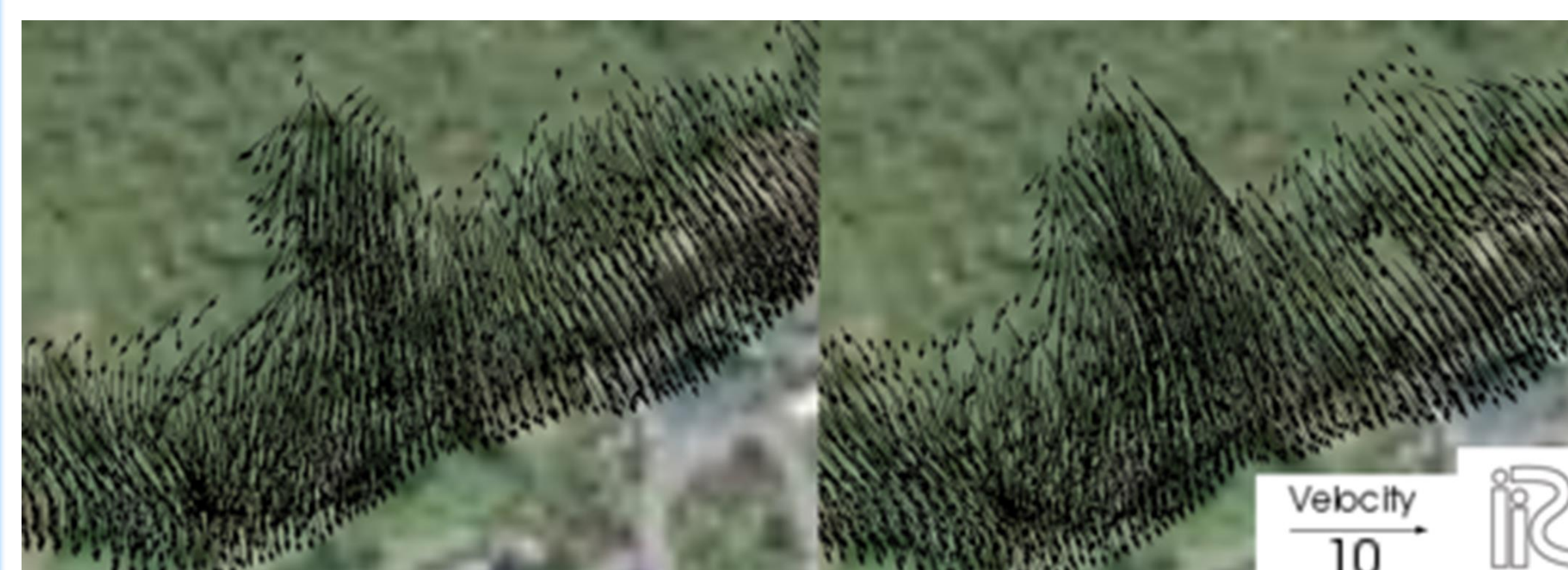
(a) Case1 (b) Case2 Fig. 4 Distribution of velocity vector after 3 seconds (unit: m/s)
