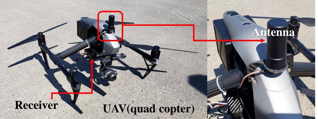
A post-processing kinematic system "Klau PPK system(Klau Geomatics)" compatible with UAV of "Inspire2(DJI)" .Electronic reference information is imported by post-processing.
