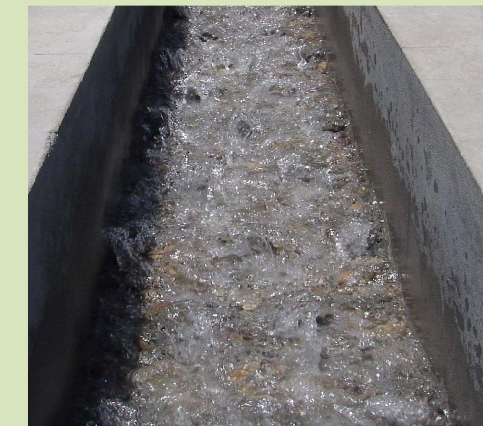
Fig.4. A typical block ramp in the experimental flume (Hydraulics Lab., CED, IIT Roorkee)
