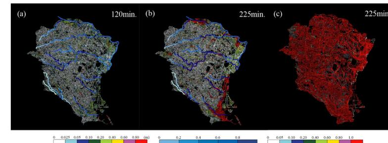
Figure 3. (a)(b) contour map of on road inundation depth at 120, 225 minutes from the beginning of rainfall, (c) contour map of drainage full rate at 225 minutes. Legend (from left): Road inundation depth, River relative water depth, Sewerage full rate.
