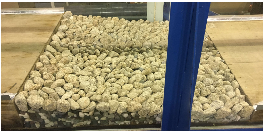
Photo 1. Installations of drop model, stacked boulders, and boards for abrupt rise in rectangular channel.
