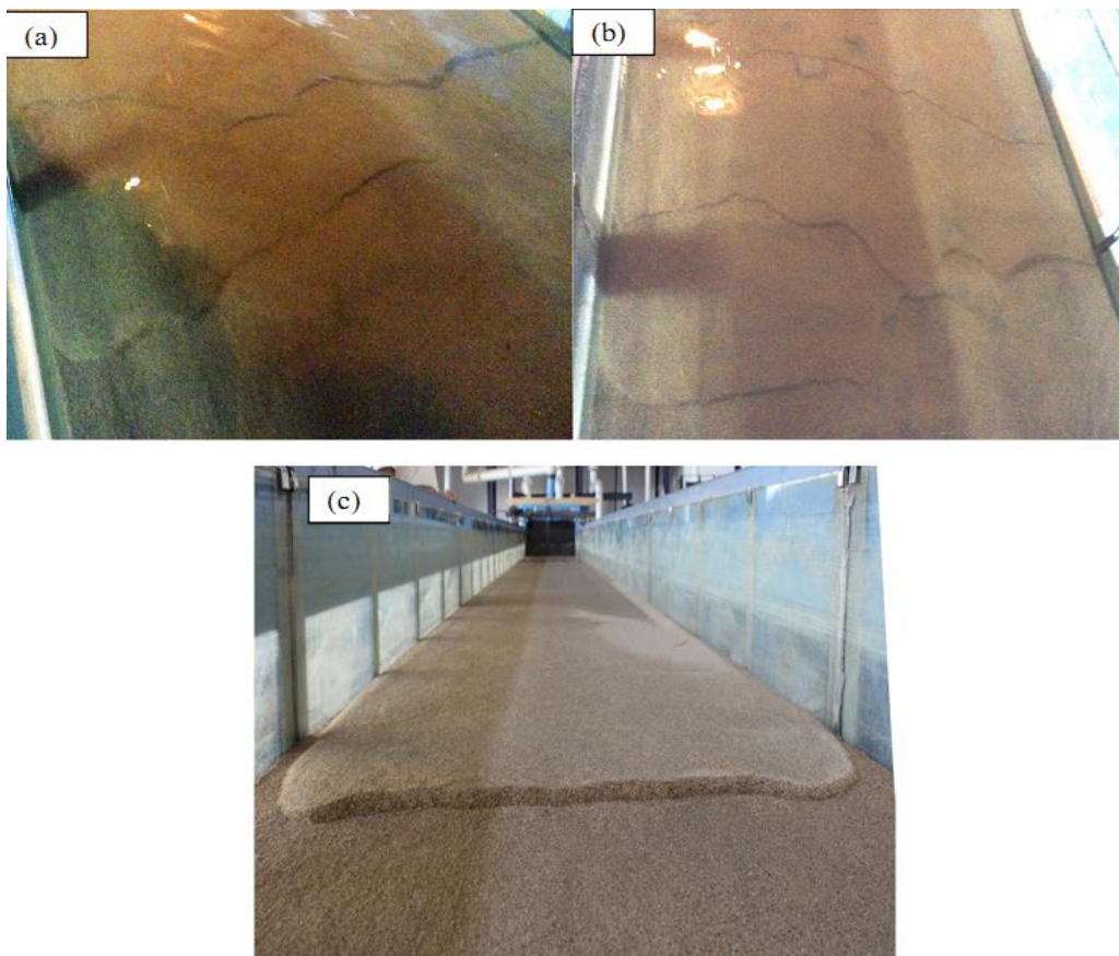
Figure 3: Snapshot of the channel (a) beginning of seepage experiment (b) during experiment (c) at the end of experiment in the seepage condition
