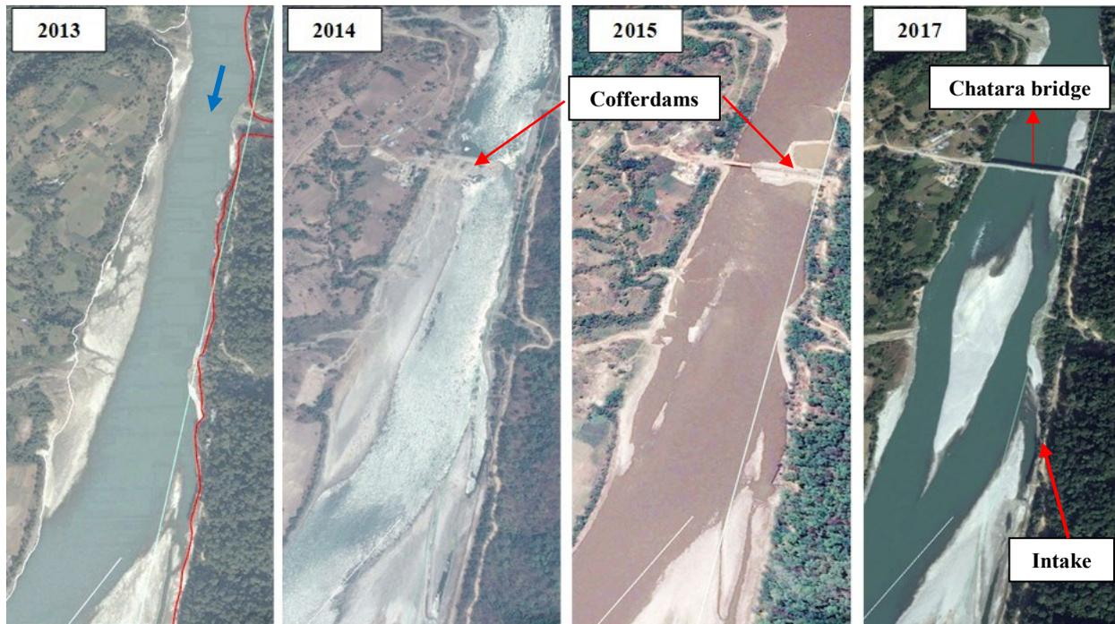
Figure 1. Google earth images showing the evolution of mid-channel bar as an effect of cofferdam
