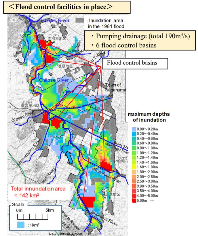
Figure 6. Simulation results for maximum depths of inundation(w/ flood control facilities)
