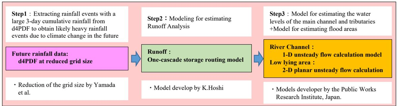
Figure 1. Schematic of the flood analysis model
