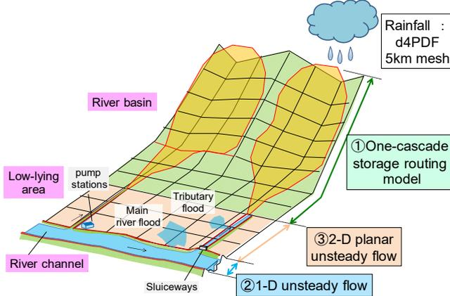
Figure 2. Flood model integrating inundation due to interior runoff and river flooding
