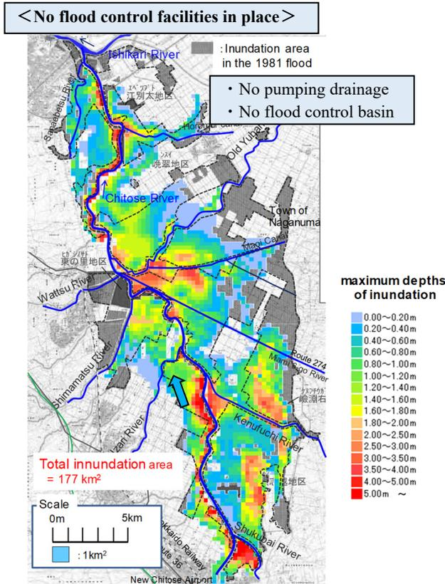
Figure 5. Simulation results for maximum depths of inundation(w/o flood control facilities)
