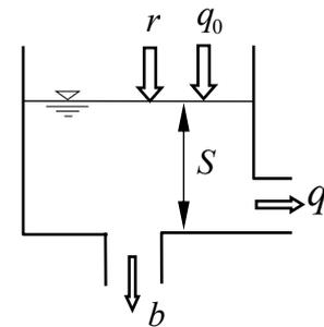
Figure 3. One-cascade storage routing model
