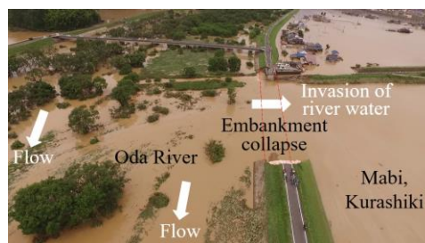
Figure 1. Breach of a levee and the vegetation flourish situation at 3.4 KP of the Oda River; where the kilometre post (KP) value signifies the longitudinal distance (km) from the river mouth (Okayama River Office, July 8, 2018).
