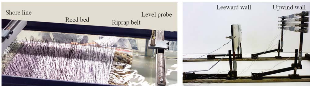
Figure 4. Left: model of the reed bed. Right: model of the breakwater with its modular metallic structure; the vertical poles are equipped with extensometric sensors at their embedding in the modelled lake bed.
