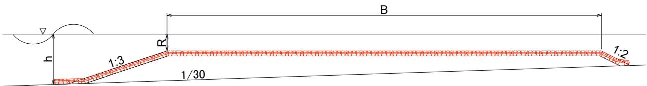
Fig.10 Cross-section of artificial reef experiment model
