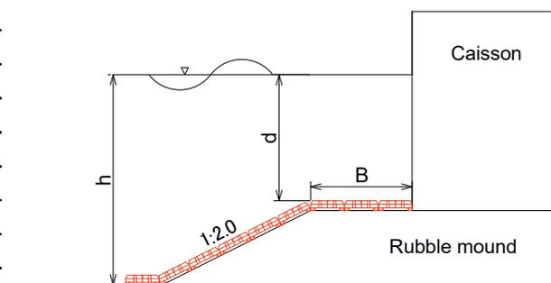
Fig.3 Cross-section of composite breakwater mound experiment model
