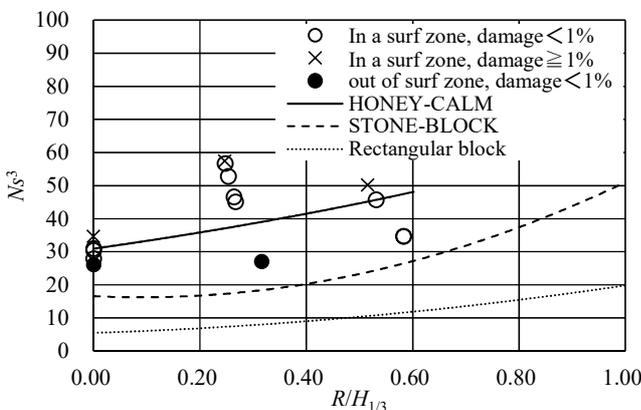
Fig.11 Experimental results of performance curve
