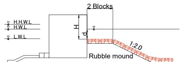
Fig.14 Cross-section of tsunami overflow experiment model
