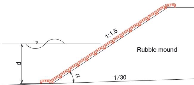
Fig.7 Cross-section of coastal dike slope experiment model
