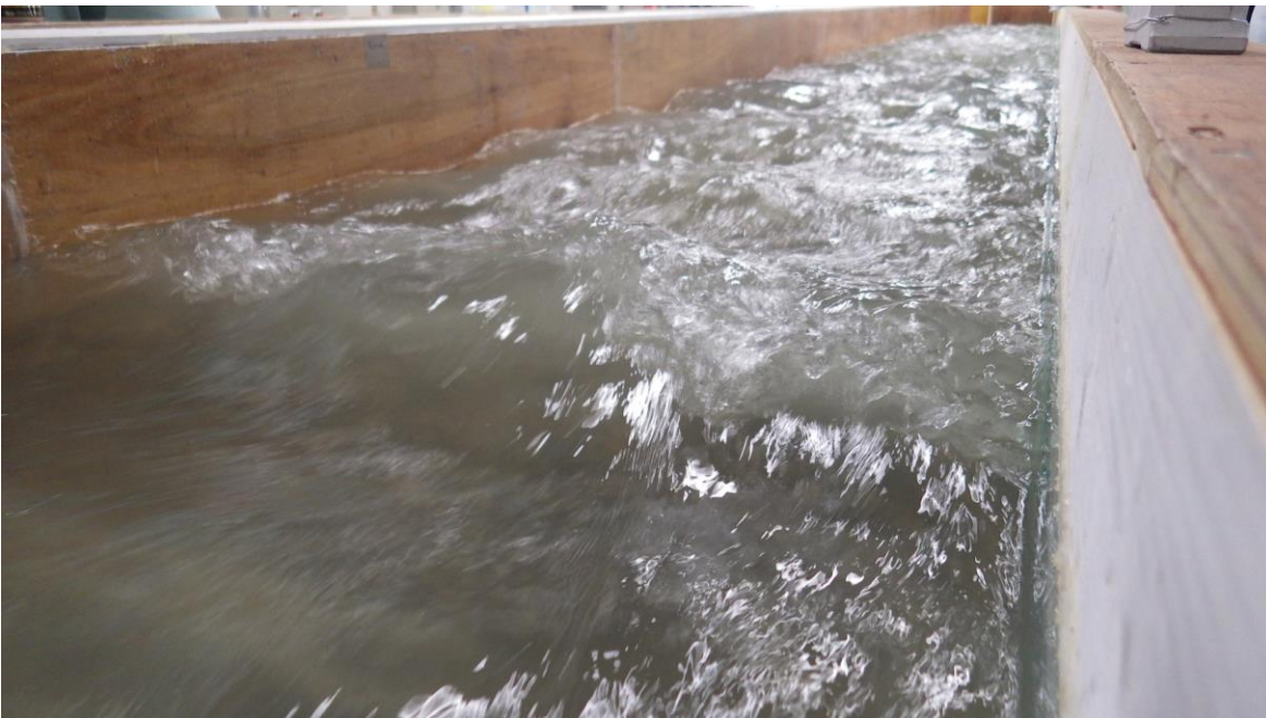
Photo 10 Flow condition during flood stage ( Q_p = 390 \text{ m}^3/\text{s} in prototype)
