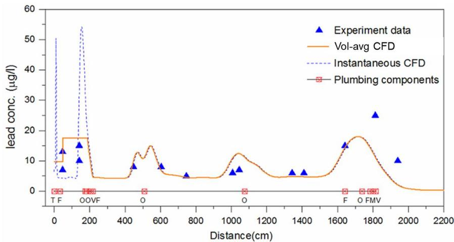
Fig. 5 Comparison of predicted and measured Pb concentration along a water supply chain; tap is turned on after 4-hr stagnation ( $Q = 80 \text{ mL/s}$ ,  $U = 0.13\text{m/s}$ ,  $Re = 3345$ ). T: tap, F: compression joint, O: solder joint, M: meter, V: valve.
