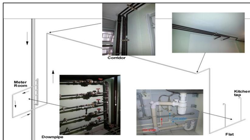
Fig. 1 Water supply system inside a high-rise building of a Public Rental Housing estate of Hong Kong.
