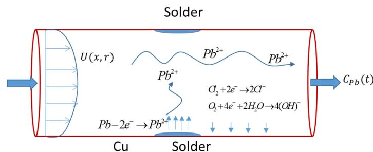
Fig. 2 Lead ( $Pb^{2+}$ ) due to galvanic corrosion and turbulent transport with flowing water to tap
