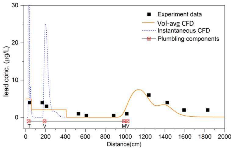
Fig. 4 Comparison of predicted and measured Pb concentration along a water supply chain; tap is turned on after 4- hour stagnation ( $Q=53\text{ml/s}$ ,  $U=0.14\text{m/s}$ ,  $Re=3800$ ): T: tap, M: meter, V: valve.
