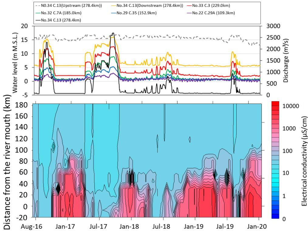
Figure 3 Electrical conductivity longitudinal heatmap, longitudinal water level, and Chao Phraya Dam discharge from August 1, 2016 to February 13, 2020 (Yusuke H. et al., 2019).
