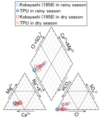
Figure 9 Trilinear diagram of data collected from No.25 C10\_T03 (131.0 km).
