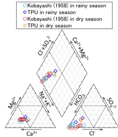
Figure 7 Trilinear diagram of data collected from No.18 C07\_S01 (water intake; 95.1km)
