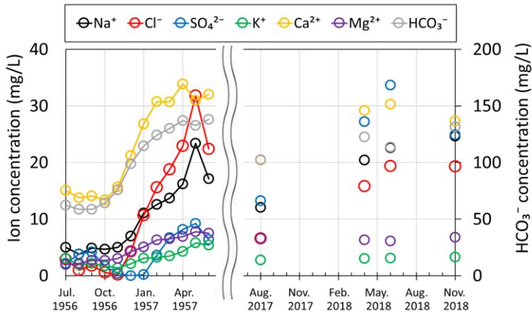
Figure 6 Time series of main ions in the river water collected at station No.18 C07\_S01 (95.1 km).
