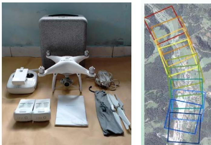
Figure 4. Drone and over-lapping/side-lapping techniques of photo aerial mapping.
