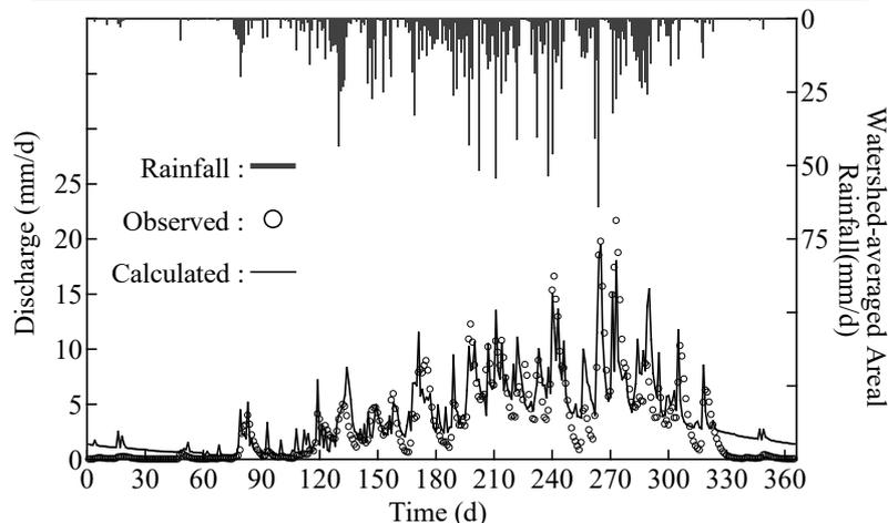
Figure 4. Comparison of the observed and calculated discharge in 2007 (NS=0.71).
