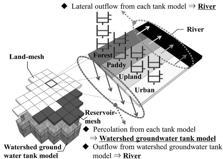
Figure 2. Structure of the distributed rainfall-runoff model.
