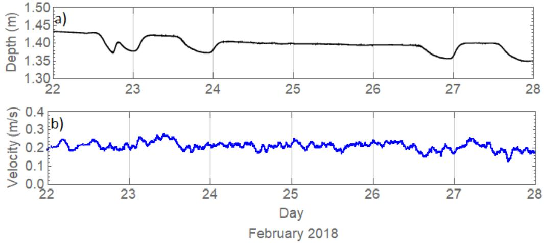
Figure 4. Temporal variations in a) average water depth (black), and b) stream velocity (blue dots).
