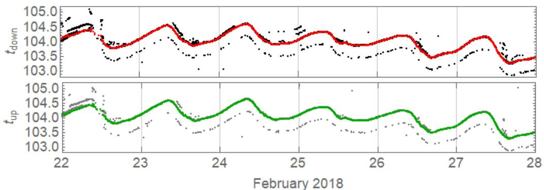
Figure 3. Arrival time (milliseconds) recorded by downstream and upstream transducers (black, and gray) and the detected inliers (red, green) by the shortest-path graph.
