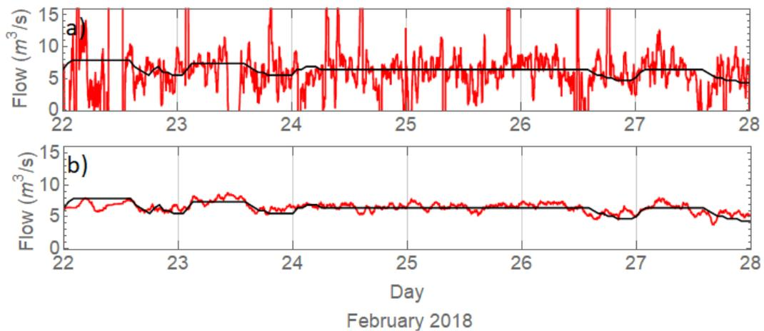
Figure 5. Discharge time series observed by FAT (red) and RC (black) during the study period a) comparison before correcting the arrival times of the acoustic transducers, and b) comparison after correcting the arrival times of the acoustic transducers using the shortest path graph.
