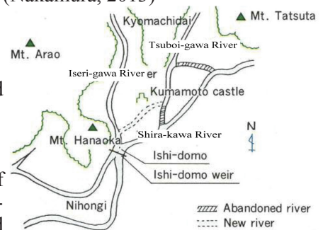
Fig.1 River improvement of the Shira-kawa River by Kiyomasa (Kumamoto River National Highway Office, 1995)
